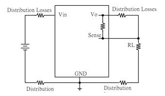
Figure 32: Effective circuit configuration for remote sense operation
