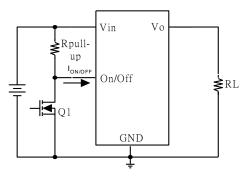
Figure 31: Negative remote On/Off implementation
