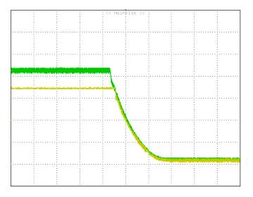
*Figure 26:*Tracking function, Vtracking=0.8V, Vout= 0.69V, full load Yellow: VOUT, 0.2V/div, Green : Tracking, 0.2V/div, 5mS/div
