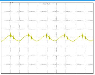
*Figure 8:* Output ripple & noise at 12Vin, 1.8V/20A out CH1:VOUT, 20mV/div, 1uS/div
