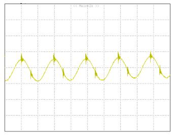
*Figure 9:* Output ripple & noise at 12Vin, 3.3V/20A out CH1:VOUT, 20mV/div, 1uS/div
