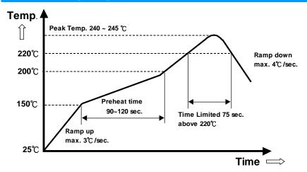
Note: The temperature refers to the pin of DCL, measured on the pin Vout joint..
