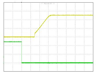
*Figure 18:* Turn on delay time at remote on 12Vin, 5.0V/20A out. (Yellow: VOUT, 2V/div, Green: ON/OFF, 2V/div, 2mS/div)
