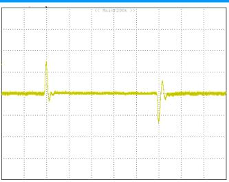
*Figure 20:* Transient response to dynamic load change at 2.5A/µS from 50%~ 100%~50% of Io, max at 12Vin, 1.8Vout (Cout = 1uF ceramic, 47uF\*2 +10µFceramic) Yellow : VOUT, 0.2V/div, 100uS/div
