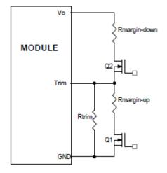
Figure 35: Circuit configuration for output voltage margining
