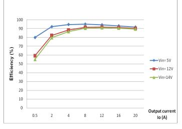
Figure 3: Converter efficiency vs. output current (1.8V out)
