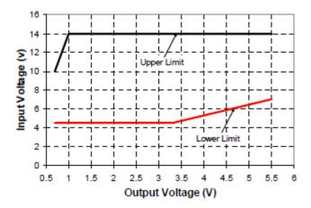
**Figure 34:** Output voltage vs input voltage setpoint area plot showing limits were the output can be set for different.input voltage.
