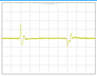
*Figure 19:* Transient response to dynamic load change at  $2.5A/\mu$ S from 50%~ 100%~50% of Io, max at 7Vin, 0.69Vout (Cout = 1uF ceramic, 47uF\*2 +10µFceramic) Yellow : VOUT, 0.2V/div, 100uS/div
