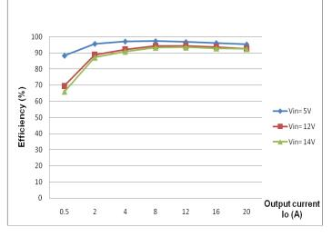
Figure 5: Converter efficiency vs. output current 3.3V out)
