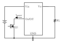
Figure 30: Positive remote On/Off implementation
