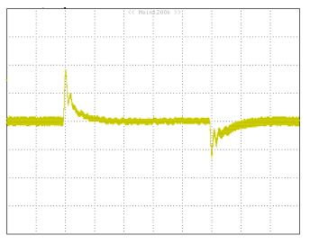
*Figure 22:* Transient response to dynamic load change at 2.5A/µS from 50%~ 100%~50% of Io, max at 12Vin, 5Vout (Cout = 1uF ceramic, 47uF\*2 +10µFceramic) Yellow : VOUT, 0.2V/div, 100uS/div
