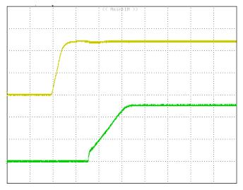
*Figure 14: Turn on delay time at 12Vin, 5.0V/20A out.* (Green : VOUT, 2V/div, Yellow: VIN, 5V/div. 2mS/div)
