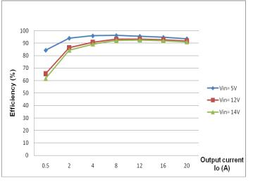
Figure 4: Converter efficiency vs. output current (2.5V out)
