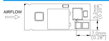
**Figure 39:** Temperature measurement location The allowed maximum hot spot temperature is defined at  $117^{\circ}C$
