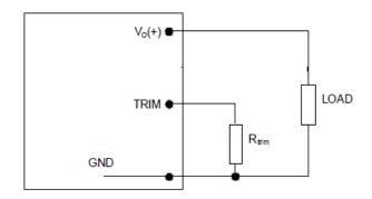
Figure 33: Circuit configulation for programming output voltage using an external resister.
