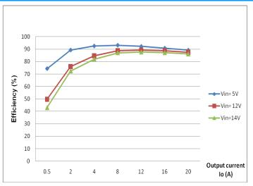
Figure 2: Converter efficiency vs. output current (1.2V out)
