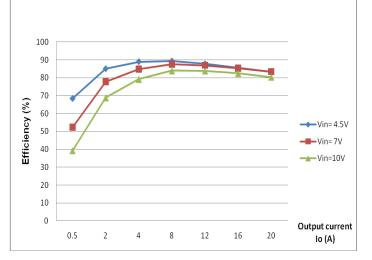
Figure 1: Converter efficiency vs. output current (Vout= 0.69V)
