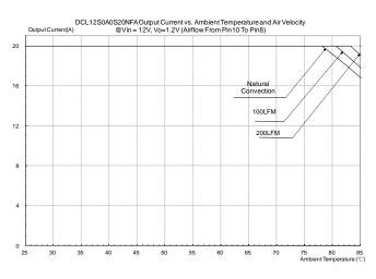
Figure 44: Output current vs. ambient temperature and air velocity @Vin=12V, Vout=1.2V(Either Orientation)
