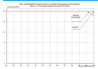
Figure 45: Output current vs. ambient temperature and air velocity@Vin=7V, Vout=0.69V(Either Orientation)
