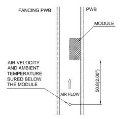
Note: Wind Tunnel Test Setup Figure Dimensions are in millimeters and (Inches)
