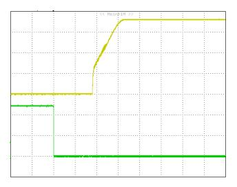
*Figure16:* Turn on delay time at remote on 12Vin, 1.8V/20A out. (Yellow: VOUT, 0.5V/div, Green: ON/OFF, 2V/div, 2mS/div)
