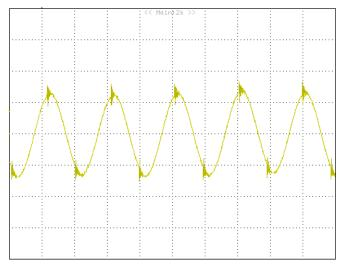
*Figure 10:* Output ripple & noise at 12Vin, 5.0V/20A out CH1:VOUT, 20mV/div, 1uS/div
