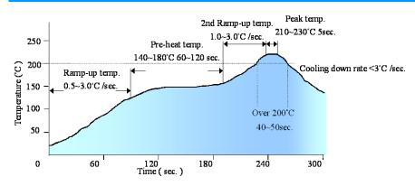
Note: The temperature refers to the pin of DCL, measured on the pin Vout joint.
