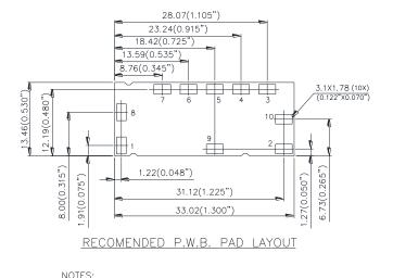
DIMENSIONS ARE IN MILLIMETERS AND (INCHES)
