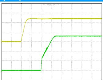
*Figure 12: Turn on delay time at 12Vin, 1.8V/20A out.* (Green : VOUT, 0.5V/div, Yellow: VIN, 5V/div. 2mS/div)
