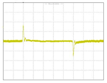
Figure 21: Transient response to dynamic load change at  $2.5A/\mu$ S from 50%~ 100%~50% of Io, max at 12Vin, 3.3Vout (Cout = 1uF ceramic, 47uF\*2 +10µFceramic) Yellow : VOUT, 0.2V/div, 100uS/div
