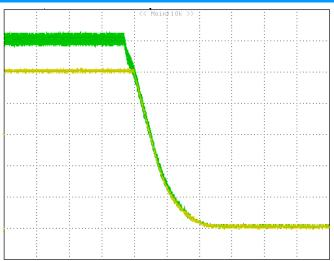
*Figure 24:*Tracking function, Vtracking=6V, Vout= 5.0V, full load Yellow : VOUT, (1V/div), Green: Tracking, (1V/div), 10mS/div
