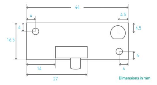
The 2 mounting holes are 3.3mm diameter.
