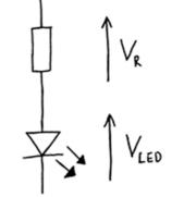
Using Ohms Law in a slightly rearranged format:
