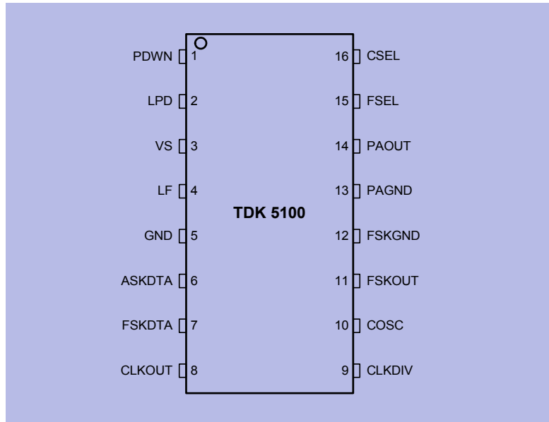
Figure 2-1 IC Pin Configuration
