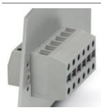
Panel feed-through terminal block, connection method: Screw connection, Screw connection, number of positions: 1, load current: 76 A, cross section: 0.5 mm² - 16 mm², AWG 20 - 6, connection direction of the conductor to plug-in direction: 90 °, width: 10.1 mm, color: gray
