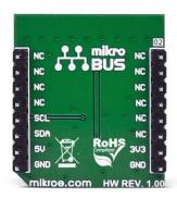
MAC Address click provides a unique node address for your application. It also has 1Kbit of writable EEPROM memory. MAC Address click carries the 24AA025E64 2K I2C Serial EEPROM with EUI-64™ node identity. The click is designed to run on either 3.3V or 5V power supply. MAC Address click communicates with the target microcontroller over I2C interface.
