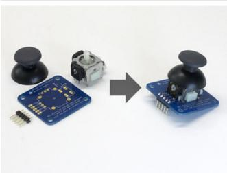
Assemble the analog thumb joystick. Some of the pins may be a little bent from shipping and need to be nudged into place. The "hat" simply presses into place.
