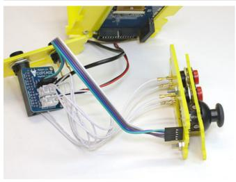
Then plug these into the corresponding sockets on the Cupcade board.
