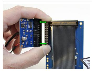
The Cupcade interface board now installs on the female header on the back of the PiTFT.
