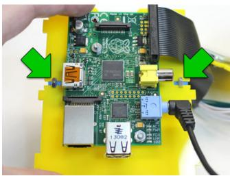
Then, from the top side, press a nut into the cross part of each "T." Give it a pinch from both sides, so the tape gets a good hold on the nut.
