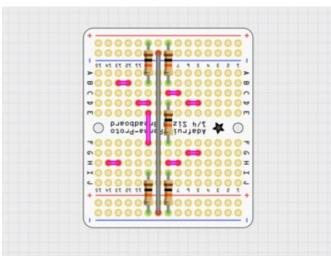
Eight short jumpers are now installed in the positions shown in pink. Most of these are very small, joining adjacent pads. We can use the un-insulated clippings from the prior step because no other conductive traces are crossed.
