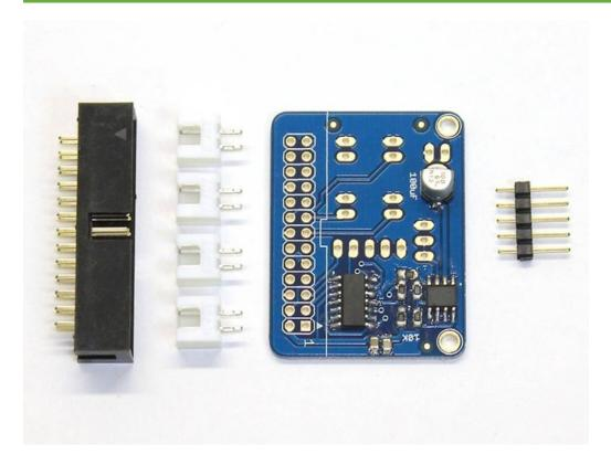
A small circuit board — specially designed just for Cupcade — features a joystick adapter circuit and a small audio amplifier. Just a few through-hole components need to be soldered.
