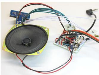
Solder the opposite end of the wires to the corresponding points on the amplifier circuit, then shrink the tubing near each end.
