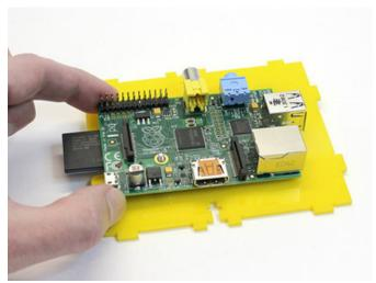
Align the mounting holes on the Raspberry Pi over these two screws.
