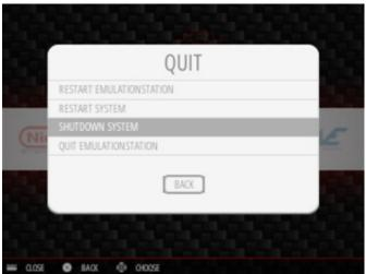
ALWAYS turn off Cupcade using the Shutdown System menu option. Just pulling the plug runs the risk of corrupting the SD card contents, and you'd have to start over.
