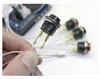
Plug a quick-connect wire set into each of the four buttons.
