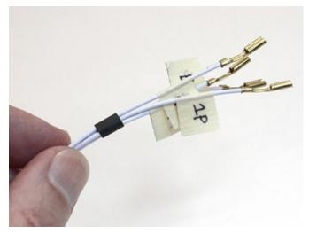
Now do a similar thing with the four *labeled* quick-connect wires. Slide a piece of heat-shrink as far along the wires as it will go.
