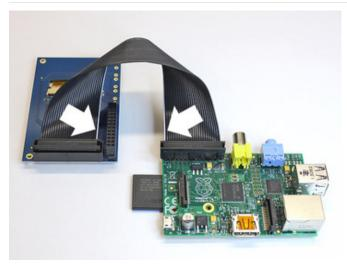
Re-install the ribbon cable between the Raspberry Pi and PiTFT, making sure the Pin 1 (white wire) is in the correct location.
