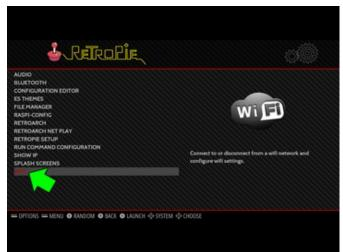
Highlight the "WiFi" option at the bottom of this list and press the A button again. This runs a WiFi configuration utility, which is all text-based...so this works with the keyboard's arrow keys, tab and enter keys to select menu items, and when asked for the network password just use the keyboard as normal.
