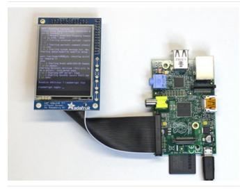
Turn the screen over and connect a USB keyboard and power. After a few seconds you should see the same bootup sequence as before. If the PiTFT worked when connected directly to the Pi but does not work with the ribbon cable:
