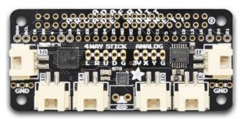
**Generation 3** (current) Cupcade kits include the **Adafruit Arcade Bonnet** with the 40-pin GPIO header as used on current Raspberry Pi boards.
