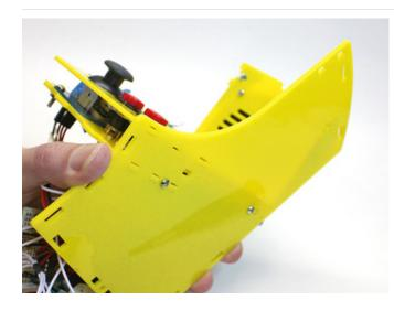
The trick now is to pick the whole thing up and feed these two screws through their corresponding holes in the side.
