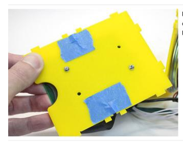
Put a piece of masking tape over each of the two T-slots on the underside of the base piece (where the Raspberry Pi is installed).
