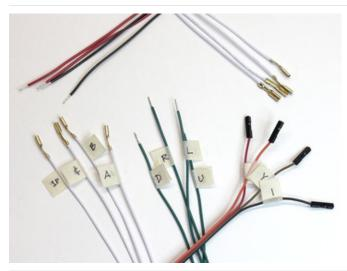
Four of the white **quick-connect** wires should be labeled with: **A**, **B**, **¢** and **1P**. The other four quick-connect wires **do not receive labels**.
