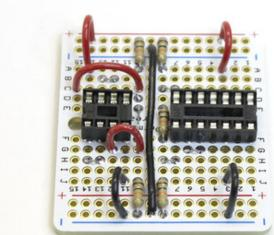
This diagram shows where the TS922 amplifier and LM339 comparator ICs will be installed later. In their place for now we'll install **sockets**, then add the chips after everything else is complete.
