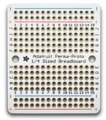
**Generation 1** kits had you solder up several components and wires on an **Adafruit Perma Proto** board.
