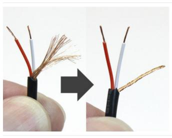
Strip 1/4" insulation from the two inner wires. Twist the stranded copper wire into a tidy bundle.
