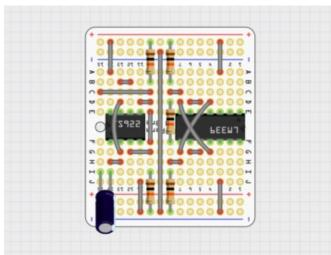
Install the 100  $\mu F$  capacitor in the position shown.
