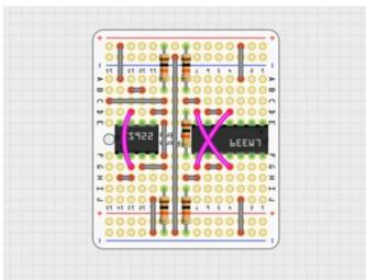
Three more jumpers are installed, cut from insulated wire.
