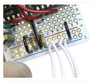
Solder the other end of these four wires to the lower ground bus on the Perma Proto board. The wires enter from the top and are soldered on the underside. Clip any excess wire protruding from the bottom.
