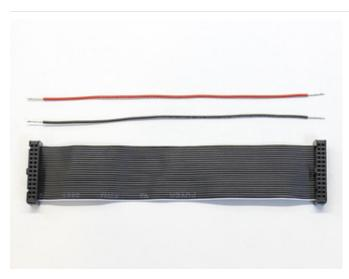
Cut two (2) wires about six inches long and strip about 1/4" of insulation from both ends.
