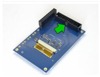
The tall female (socket) and shorter male (pin) headers will be installed in the positions shown. The female socket goes on the long edge of the PiTFT board, male on the short edge (labeled "Connector on reverse!" on the silkscreen side of the board).
