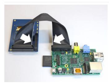
The header on the PiTFT is "keyed" so that pin 1 (the white wire) is always on the correct side. However, there's two ends to the cable. Plug in the end that places the cable running behind the PiTFT board, not out in the open.
