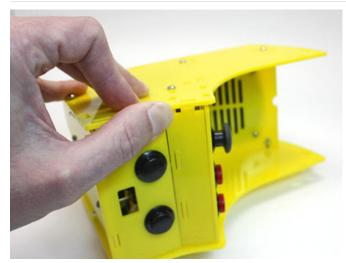
Install this fascia piece in a similar manner, then tighten the side screw back as it was.
