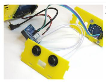
Plug the ¢ (left) and 1P (right) buttons into the corresponding sockets on the Cupcade board.
