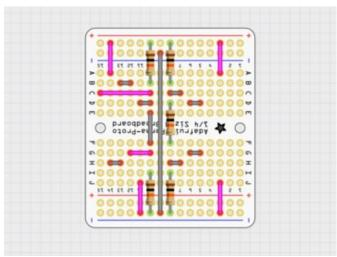
other traces, they should be cut from **insulated** wire,  $\underline{\text{do}}$  not use the resistor clippings for this step!
