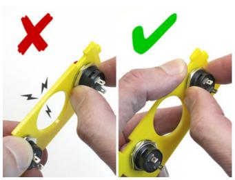
Two red buttons are installed on the chosen control cutout. Because this part is thin in one spot, it must be done with care.
