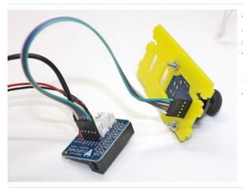
Connect the female jumper wires between the joystick and Cupcade board, making sure you get the same sequence (e.g. GND to GND and so forth). If you get these out of sequence, the Pi might not boot!
