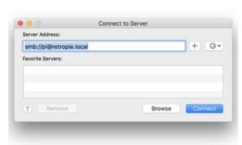
Here's how one typically connects from a Mac, using the Finder's Go→Connect to Server... option. Windows, Linux will have their own equivalent functions.
