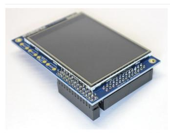
This is what good soldering looks like. The solder flows smoothly between the pins and the pads on the board, no blobs, bridges or gaps. The Adafruit Guide to Excellent Soldering (https://adafru.it/cA6) has pointers for novices.
