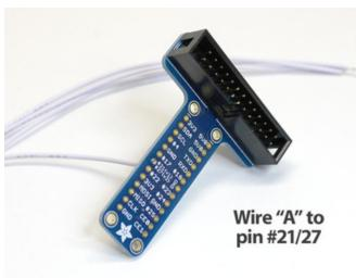
Using the schematic at the top of this page for reference, solder the other end of the wire to the appropriate point on the T-Cobbler. Wire A goes to Pin #21/27
