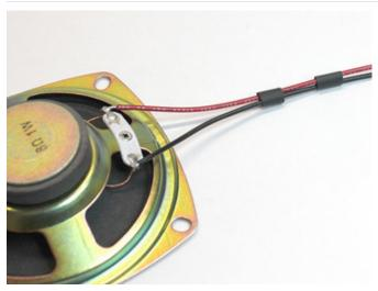
Solder one end of these wires to the connection points on the speaker.
