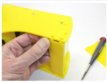
Slot the marquee into place, then re-tighten the top screw.
