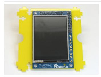
Install the PiTFT on its backing piece using three tiny #2-56 screws and matching nuts.
