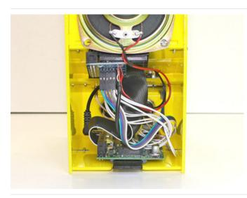
Stuff the wires into the back of the case, being careful not to dislodge the Cupcade board.
