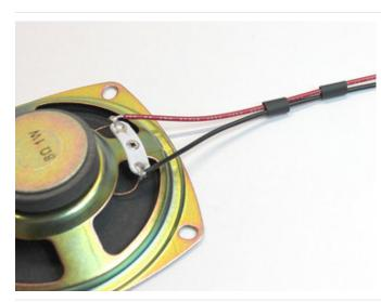
Solder two plain wires to the connection points on the speaker.
