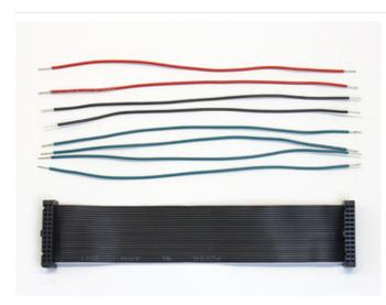
Cut eight (8) wires about six inches long and strip about 1/4" of insulation from both ends.
