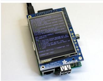
Install the PiTFT on the Raspberry Pi, making sure the header pins are aligned.
