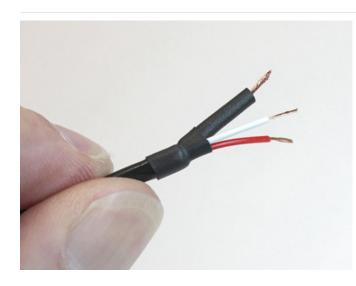
That bare copper wire on the audio cable is a problem... it connects to a ground point *right next* to a +5V line. **We must insulate!**
