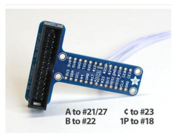
Repeat with the other three wires, <u>one at a time</u> so you don't get them mixed up. Slide one wire part way out of the heat-shrink, grab the "tail" and solder in to the correct spot:
