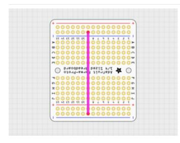
The Perma-Proto is turned around, with the labels upside-down. It's fine, this orientation just makes our circuit easier to lay out.
