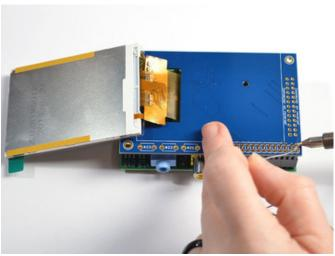
When soldering the female header, the Raspberry Pi can be used as a "stand" to hold the header and board in alignment. For the male header, you'll probably need to hold it in place temporarily with masking tape.
