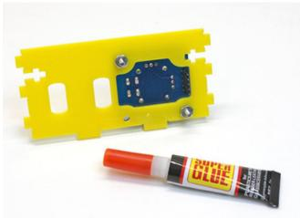
Install the joystick on its support piece, whichever one you selected (centered or off-center). Two screws at opposite corners are sufficient.
