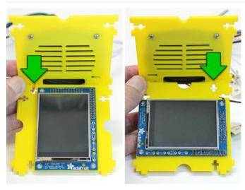
The screen fits into two slots at the bottom of the speaker grille.
