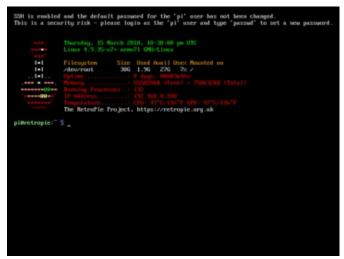
One option is to type commands directly on the Pi. From the RetroPie main screen, press "F4" to exit the GUI and get a command line prompt. From here, you could test the network connection by typing:
