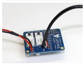
The speaker and headphone wires then connect to corresponding points on the board. The speaker wires go to the two "Spkr" points, headphone to the three "Audio" points: red wire to "R," black or white wire to "L," copper wire to "GND."
