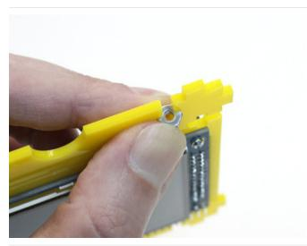
Feed a nut into the cross part of the "T," holding it in place between thumb and forefinger.
