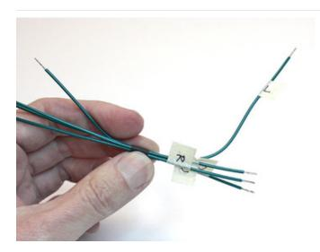
It's a very similar game with the U/D/L/R wires: squeeze them all through a piece of heat-shrink tube, then pull out one wire at a time, soldering the tail (unlabeled) end to the appropriate locations on the Cobbler...
