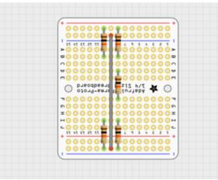
Install five **10K resistors** (brown-black-orange) in the positions shown, immediately to the left and right of the ground wire. Two go on the left (audio) side, three on the right (joystick) side.
