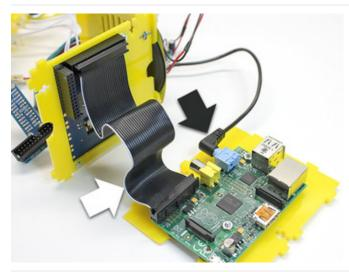
Plug the audio cable into the headphone jack and the ribbon cable to the GPIO header, making sure pin 1 (the white wire) is in the correct place.
