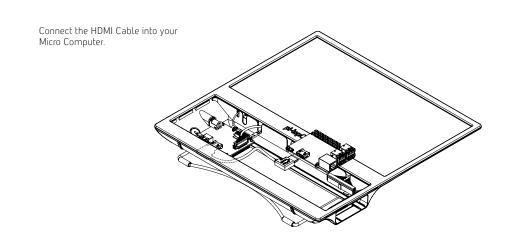
Step 5: Inserting Micro Computer
