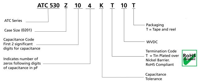
The above part number refers to a 530 Series (case size Z) 100 nF capacitor, K tolerance (±10%), with T termination (tin plated over nickel barrier, RoHS compliant), 10 WVDC, tape and reel packaging.
