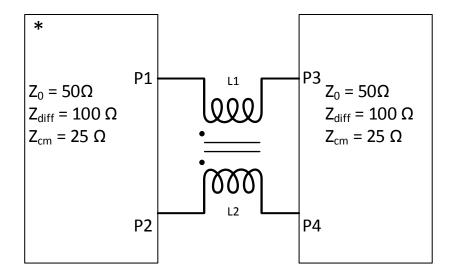
\*ENA Network analyzer E5071B/C or equivalent
