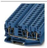
Feed-through terminal block, Connection method: Spring-cage connection, Cross section: 0.2 mm<sup>2</sup> - 16 mm<sup>2</sup>, AWG: 24 - 6, Width: 10.2 mm, Color: blue, Mounting type: NS 35/7,5, NS 35/15
