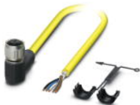
Sensor/Actuator cable, 5-position, PVC, yellow, shielded, free cable end, on Socket angled M12 SPEEDCON, A-coded, Cable length: 10 m
