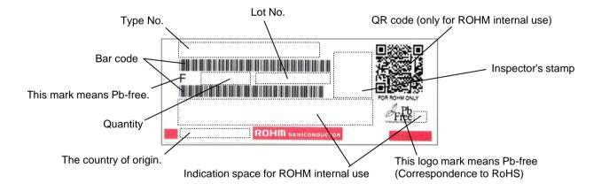
9. Type Product code of taping shall be composed as indicated below.
