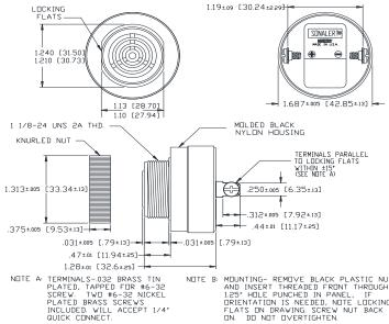
NOTE B: MOUNTING- REMOVE BLACK PLASTIC NUT AND INSERT THREADED FRONT THROUGH 1.25' HOLE PUNCHED IN PANEL, IF DRIENTATION IS NEEDED, NOTE LOCKING FLATS ON DRAWING. SCREW NUT BACK ON. DO NOT DVERTIGHTEN.
