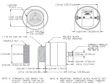
NOTE A: TERMINALS-.032 BRASS TIN PLATED, TAPPED FOR #6-32 SCREW. TWD #6-32 NICKEL PLATED BRASS SCREWS INCLUBED. WILL ACCEPT 1/4\* QUICK CONNECT.
